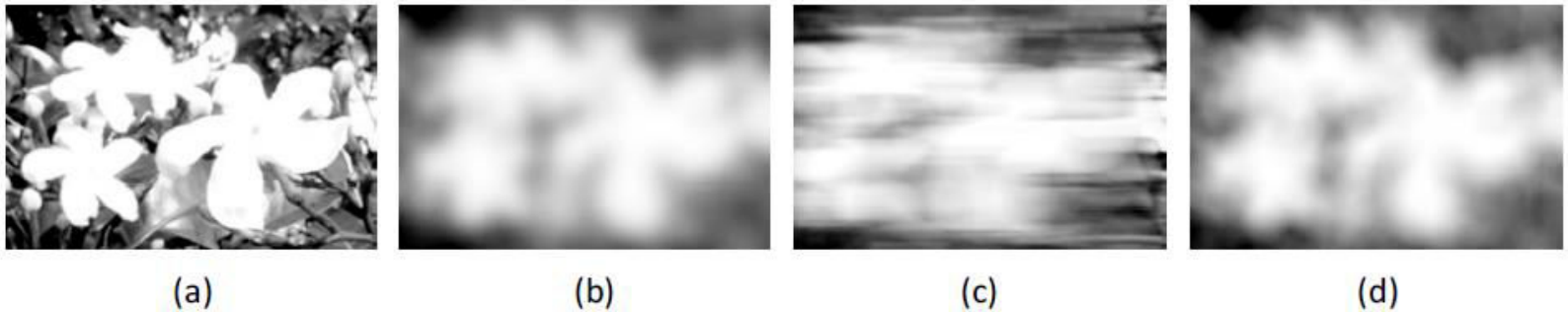
Fig. 6.3 Effect of blur (a) Original image (b) Image with Gaussian blur (c) Image with motion blur (d) Image with lens-out-of-focus blur
